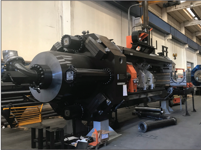
Figure 5. The 28 MN extrusion press under construction in Italy.
